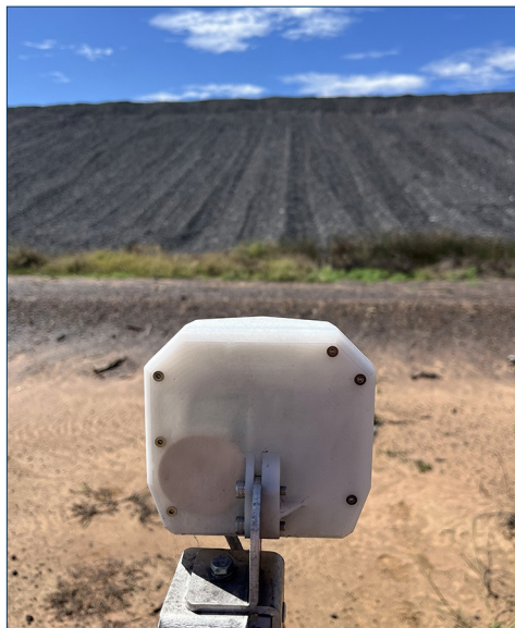
Thirteen NanoRadar units, spaced approximately 400 feet apart, were deployed to monitor this tailings embankment. Measurements were transmitted to a Starlink WiFi network and relayed to a project website.
